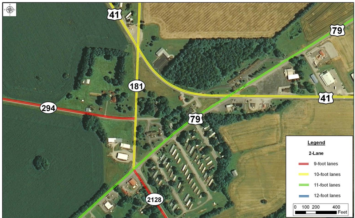
Figure 3: Lane Widths on Study Area Roadways
